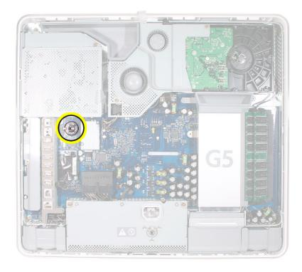
4. With a flat-blade screwdriver, plastic tool, thumb, or finger, push the battery in the direction of the arrow to free the battery from the metal clip.
